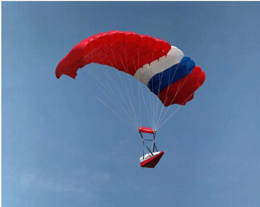
Figure 1.1: NASA Spacewedge subscale model being delivered using a steerable parafoil in 1992 during a flight test.
