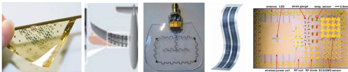
Figure 2. Sub-systems built on flexible layers: electronics, actuation, antenna, and solar cells; epidermal electronics (rightmost) integrate several of them in the same thin, peelable layer.
