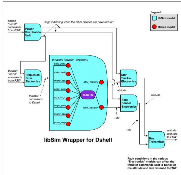
Figure 3: DSHHELL wrapped by LIBSIM
