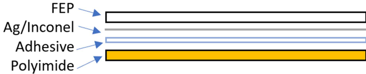
Fig. 3 Illustration of zero-pressure balloon bi-laminate film material lay-up.
