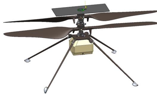
**Fig. 3 CAD drawing of the Mars Helicopter**
