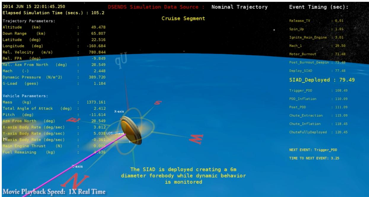
Figure 17. LDS/ SIAD Telemetry Visualization Using DSENGS
