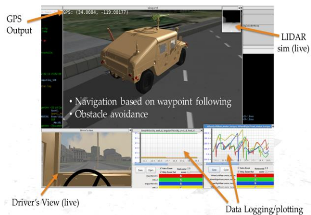
Figure 9: Scenario 1 - Urban driving with navigation and obstacle avoidance. From the top left of the figure going clock-wise, note these features: (a) GPS output, (b) the simulated LIDAR output is shown in gray levels, (c) data logging records and plots various vehicle telemetry, (d) a sample driver's view.
