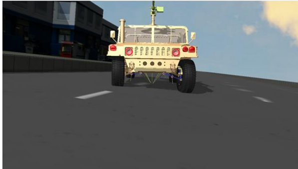
Figure 10: Scenario 2 - Lane change maneuver: Note the roll of the vehicle as it changes lanes
