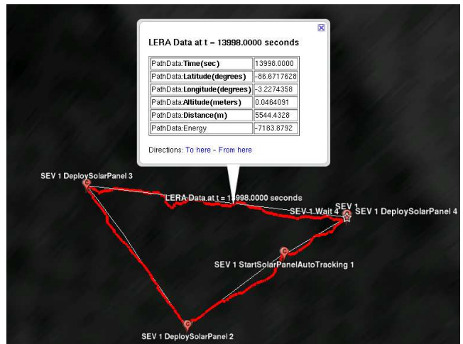
Figure 8: A view of the KML file generated from the logged simulation data overlaid on top of the LSOS KML plan.
