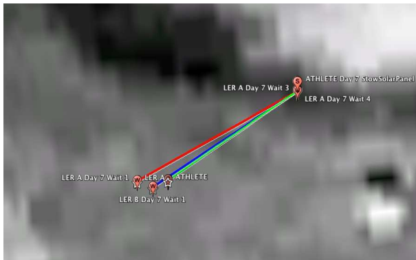
Figure 11: A view of the mission plan and analysis overlay for two simulated SEV rovers and one ATHLETE robot during one day of the Lunar traverse experiment. The red line indicates the simulated path of the SEV “A” rover, the blue line shows the simulated path of SEV “B” rover, and the green line shows the simulated path of the ATHLETE rover.
