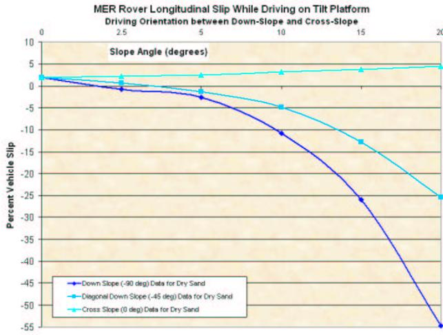
Figure 7. DTM downhill mobility test data
