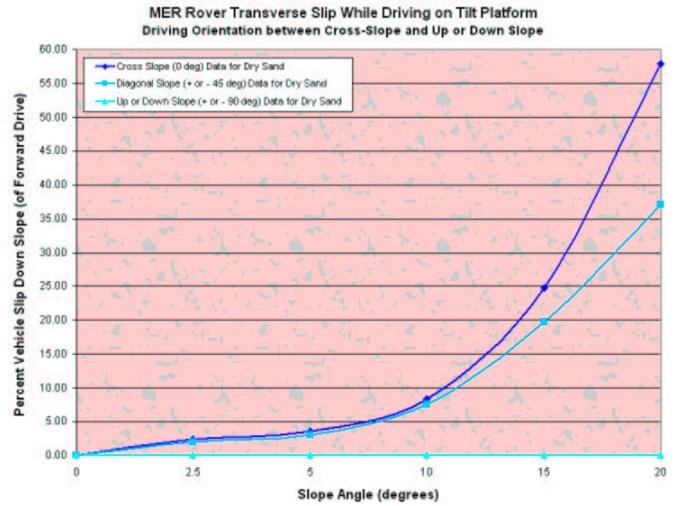
Figure 8. DTM cross-hill mobility test data
