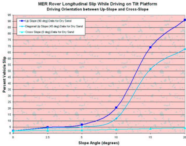
Figure 6. DTM uphill mobility test data
