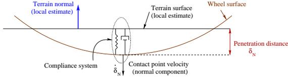
Figure 4. Normal direction compliance system
