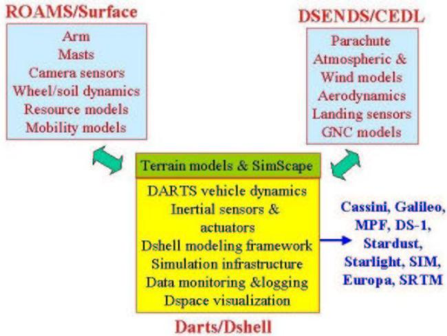
Figure 2. Common Dshell simulation infrastructure for ROAMS and DSEDS
