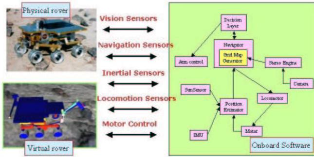
Figure 1. Typical closed-loop interfaces between on-board software and the physical/simulated rover
