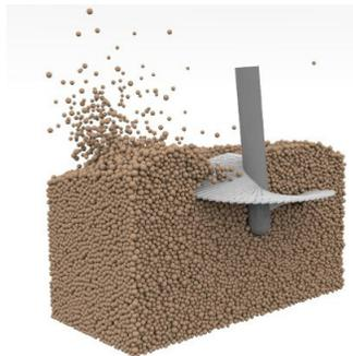
(b) Cutaway view: Anchor penetrating granular material [18].
