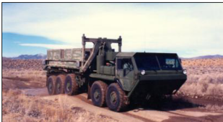
Figure F-1: LVSR-TD 10 x 10 Prototype During Ride Quality Testing.
