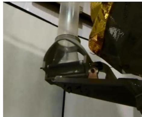
Figure 14: Detail of pinch-roller winch on Option A capture testbed
