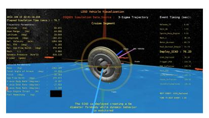
**Figure 4. ETV Supporting LDSD Flight Simulation.** ETV receives mission telemetrey data and displays vehicle state and health using polygon-based 3D spacecraft and environment representations, as well as run-time updated tabular data and ornamental CAD items such as compass graphics, velocity and line-of-sight vectors.
