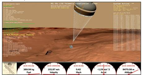
Figure 5 - MSL EDL Visualization Tool based on the new DSENDS used in MSL Mission Control during Mars Entry, Descent, and Landing
