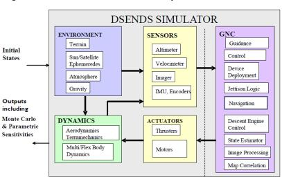
Figure 3 - DSENDS Functional Block Diagram
