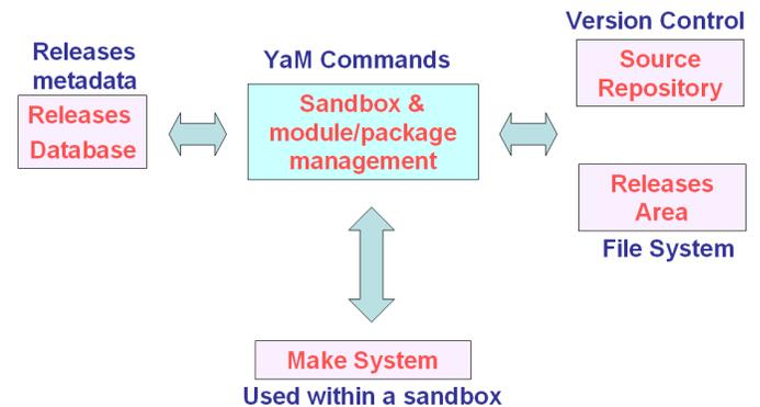
Fig. 3. The key components of **YAM** include a source repository, a database for releases data, and Perl for command line scripts.
