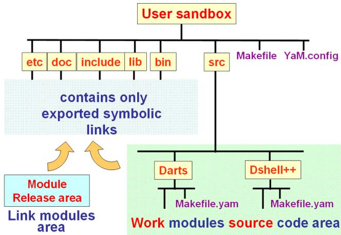
Fig. 7. The structure of a typical YAM sandbox.
