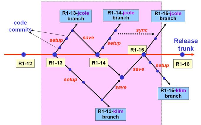
Fig. 5. The software development proceeds through a continual series of branch, develop, merge and integration cycles. The **YAM** commands in the figure are described in Sectino II-A.
