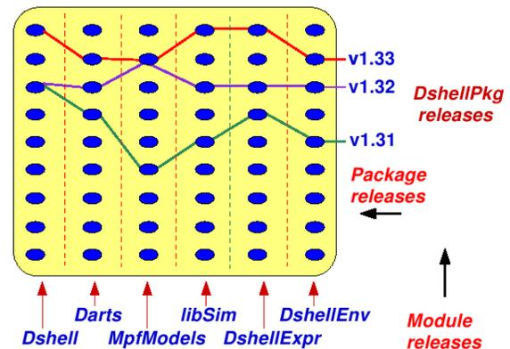
Fig. 6. The module release area hosts built versions of the releases of all the modules. Each column represents a module and the entries in the column the different releases for the module. package releases on the other hand are the lines that run horizontally across the modules and define specific module releases that belong to a package release.
