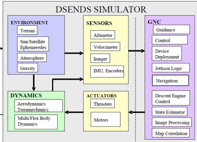
Figure 3 - DSEENDS Functional Block Diagram
